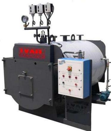
*Steam boiler monobloc, with reverse flame (pressurized combustion), pressure 11.8 bar (on request also 14.7 bar), high efficiency, equipped with wide furnace with wet back, dry saturated steam thanks to an effective humidity separator placed before the outlet. Easy maintenance thanks to the big front door and to the bolted smoke chamber totally dismountable. Suitable to work with gas, oil or heavy oil. Partially exonerable from the qualified conductor up to mod. BHP 3000 (3000 kg/h of steam).*
